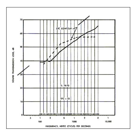
The sound transmission loss of the tested specimen is shown by the curved line in the above graph. The broken line is the limiting sound transmission class contour.
